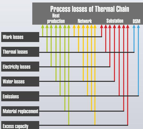
An efficient building level substation has a positive impact on most losses. Life Cycle savings of 25% on operating cost can be expected by modernizing networks with high-tech substations.
